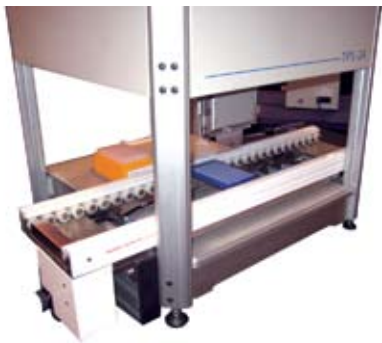
BioTrack integrated to liquid handler deck.
