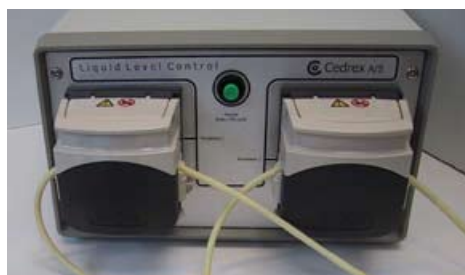
Fill and Drain pumps.
