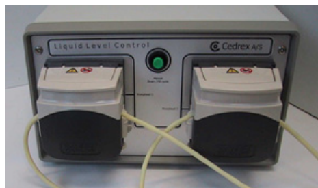
Fill and Drain pumps.
